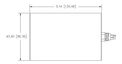
Dimensions above shown for 7km depth rated DC powered light.
